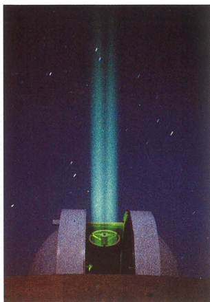
Laser ranged on the Moon by a 1.50 m telescope.
