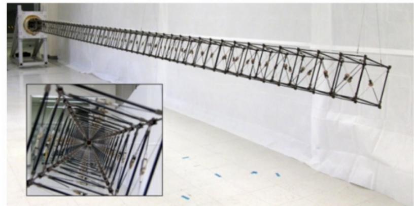
deployable mast which extends to 10.14-m after launch
